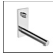
HANSASIGNATUR Electronic washbasin mixer for wall mounting, DN 15, Mains operated with thermostatic temperature mixing 4491 2010 chrome, sensory electronic operation projection: 195 mm
