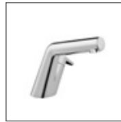
HANSASIGNATUR One-hole single-lever washbasin mixer, DN 15 with pull-out shower hose 5505 2281 chrome push pop-up waste, connection via flexible pressure hoses G 3/8, Spout swivelling, 150°, projection: 168 mm
