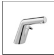
HANSASIGNATUR One-hole single-lever washbasin mixer, DN 15 5501 2201 chrome push pop-up waste, connection via flexible pressure hoses G 3/8, Spout swivelling, 150°, projection: 168 mm
