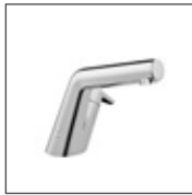
HANSASIGNATUR One-hole hybrid washbasin mixer, DN 15 Battery operated with pull-out shower hose 5510 2281 chrome, push pop-up waste, connection via flexible pressure hoses G 3/8, Spout swivelling, 150°, projection: 168 mm
